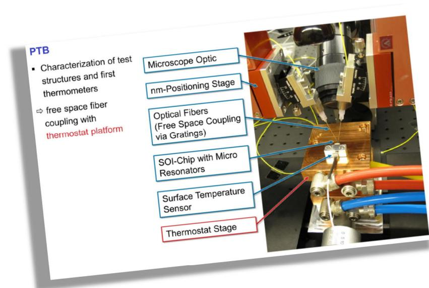
PTB thermostat for validation of photonic devices
